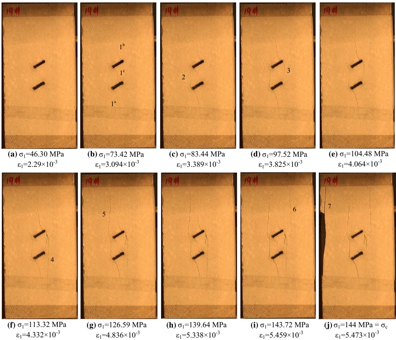
Fig. 11 Crack initiation and coalescence process of sandstone specimens containing two non-coplanar fissures for \beta = 120^\circ
