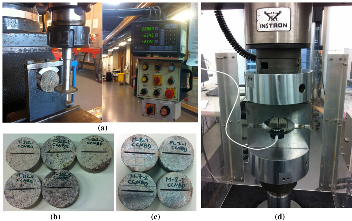
Fig. 3 CCNBD specimen preparation and experimental setup of CCNBD test according to ISRM suggestions
