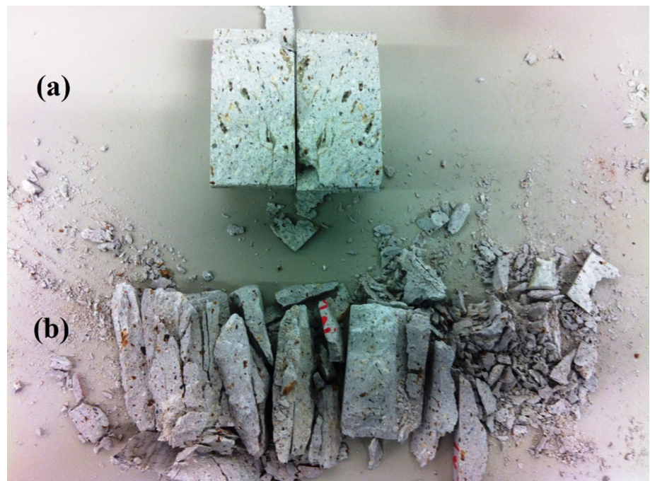
Fig. 11 Density of micro-fracture in front of the notch crack in a CCNBD specimen under, a static loading and b cyclic loading
