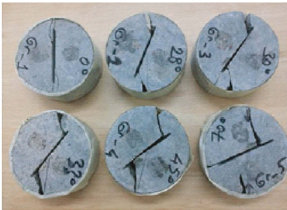
Fig. 7 Photo of recovered CCNBD samples under mixed mode loading (reproduced after Erarslan and Williams 2013)
