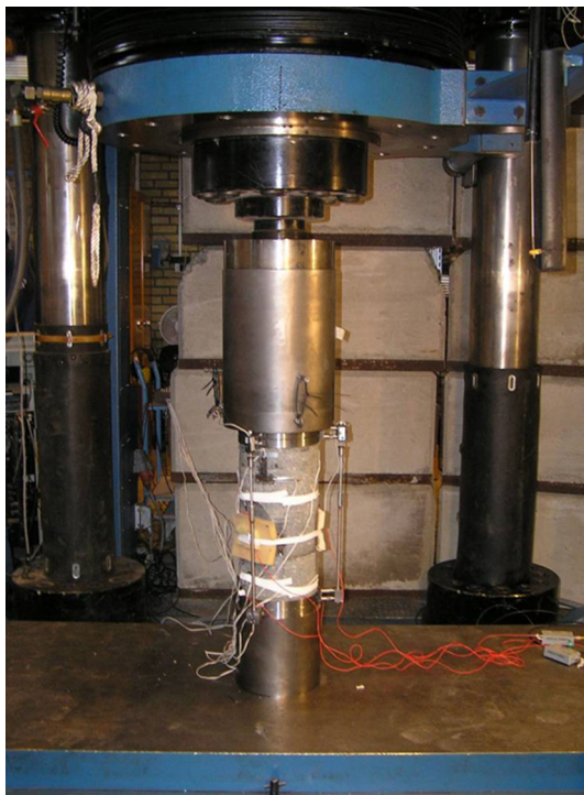
Fig. 9 Specimen KS0044B02 placed in the load frame right before testing. The concrete blocks sealing off towards the control area are seen in the background
