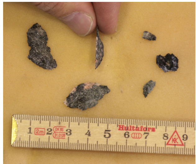
Fig. 15 Chips that have fallen off specimen KS0044B02 from side 1. The pieces are up to 25–28 mm long, thickness/depth about 5 mm
