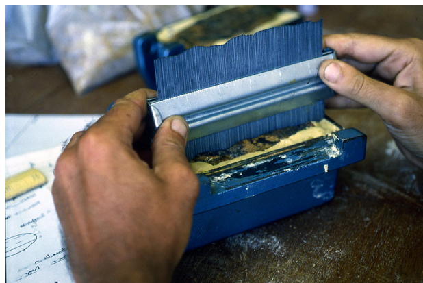
Fig. 11 Decorator’s profile gauge being used to record roughness. The device and method are sufficiently precise for recording and characterising the overall nature of the joint for geological and geotechnical characterisation
