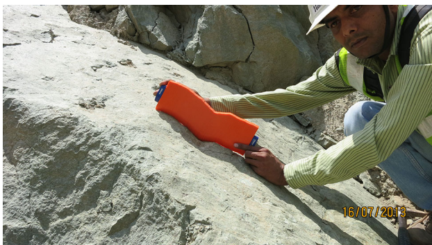
Fig. 35 Second order roughness being characterised using pin profiler
