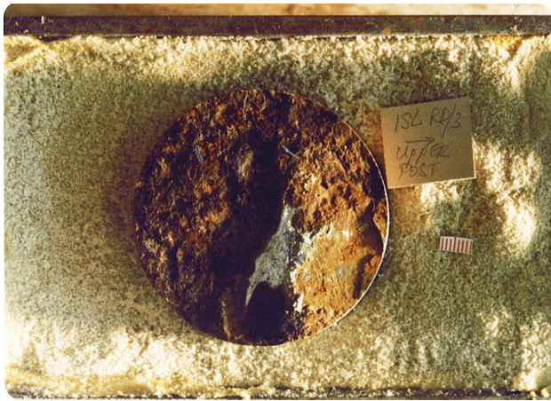
Fig. 25 Intact rock bridge ( light area ) in an otherwise weathered joint through volcanic tuff (from Hencher 1984)
