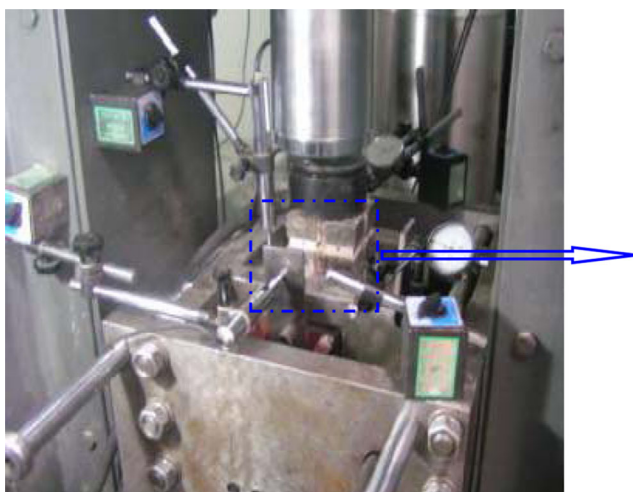
Fig. 2 True triaxial loading-unloading device
