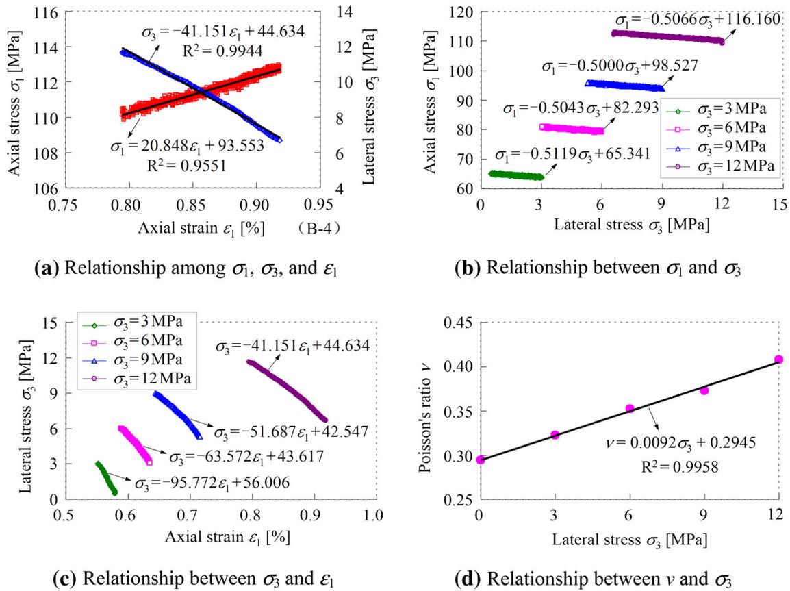
**Fig. 2** Relationship between stress and strain of the loading axial stress and unloading lateral stress triaxial tests
