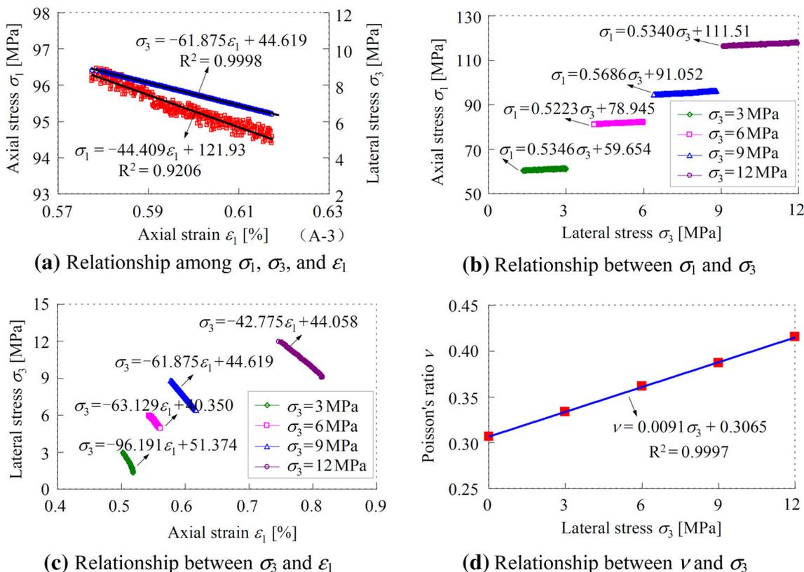
Fig. 1 Relationship between stress and strain of unloading axial and lateral stress triaxial tests
