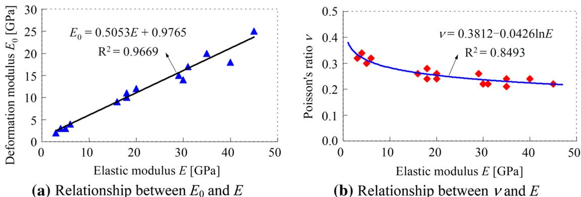
**Fig. 3** Diagrams of the mechanical parameters of Baihetan hydropower station basalt
