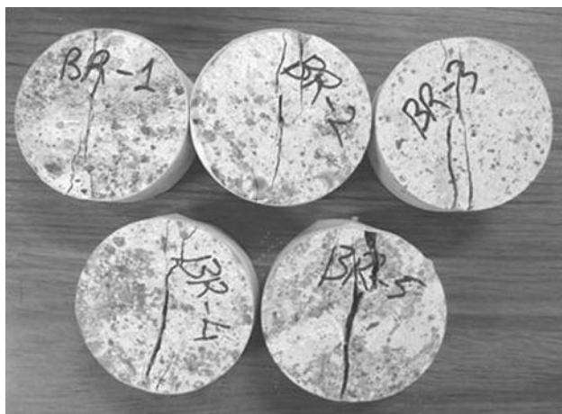
Fig. 8 Observed failure modes in the Brazilian test on Brisbane tuff (after Erarslan and Williams 2012b)
