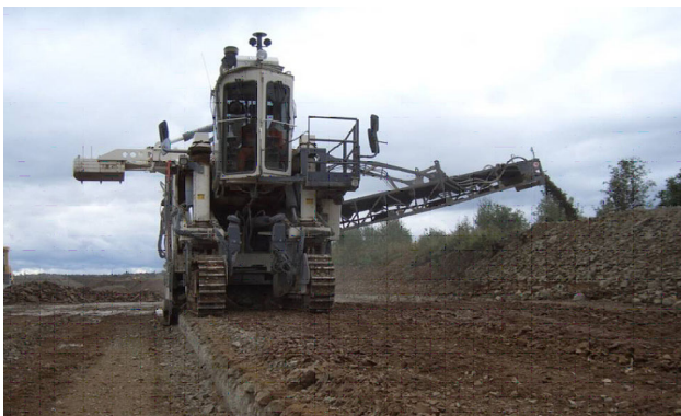
Fig. 1 An example of a surface miner ( http://www.wirtgen.de/en/produkte/surface_miner/ )
