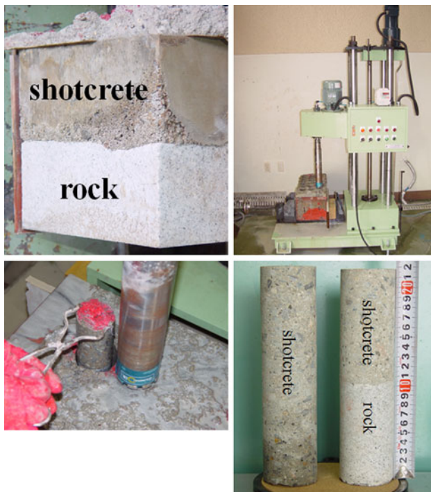
Fig. 4 NX coring for test specimens
