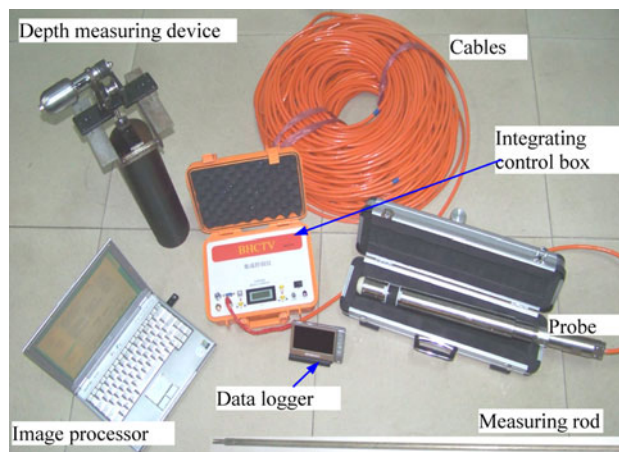
Fig. 1 The basic components of a typical borehole digital optical camera system. Note the photo of the components may change in case of the different borehole digital optical camera system
