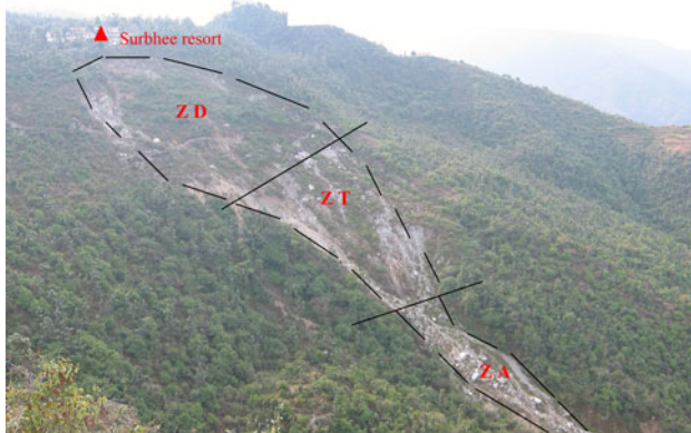
Fig. 3 Overview of Surabhi Resort Landslide. Black lines indicate the track length of 3.5 km
