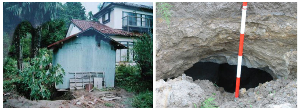
Fig. 18 Caving at Yamoto abandoned mine (from Aydan and Kawamoto 2004)
