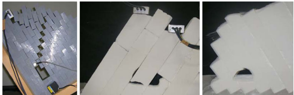
Fig. 6 Views of some model tests in discontinuous rock mass models
