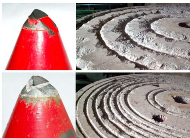
Fig. 2 Grooves with new ( top ) and worn bit ( bottom )
