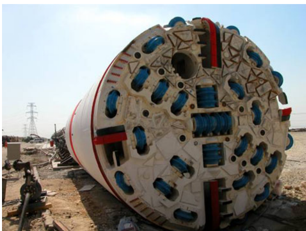
Fig. 4 Double shield TBM at the ET portal
