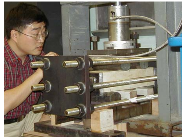
Fig. 6 Experimental setup to simulate spalling using an axially compressed beam subjected to bending
