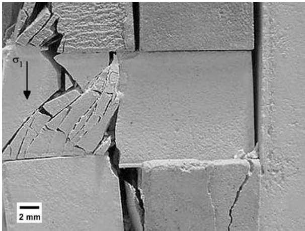
Fig. 18 Shearing fracture passing through a series of tensile cracks
