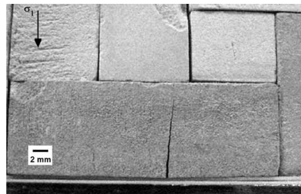
Fig. 13 First tensile cracks observed in the lengthy horizontal elements
