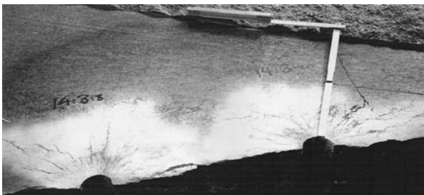
Fig. 1 Characteristic fracture pattern around \text{\O}64\text{-mm} blastholes in granitic rock (from Olsson and Bergqvist 1995). The explosive type used was Kumulux 22. The fractures are of different lengths, shapes and sizes, and the estimated thickness of the damage zone was 25 cm
