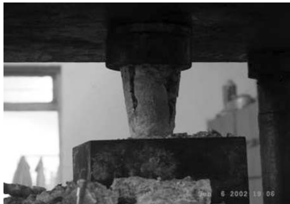
Fig. 4. Photo of cylindrical sample failure in uniaxial compression test at 120 °C
