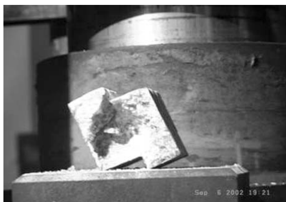
Fig. 8. Photo of failure sample of the salt rock in pre-set angle shear test at 120^\circ\text{C} with angle \alpha of 40^\circ
