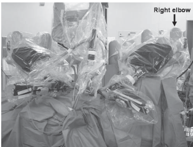
Fig. 2. Positioning of the da Vinci surgical system for robotic internal thoracic artery harvesting. It is very important to face the elbow of the robot arm toward the outside as much as possible to avoid conflict between the robotic arm and the camera arm
