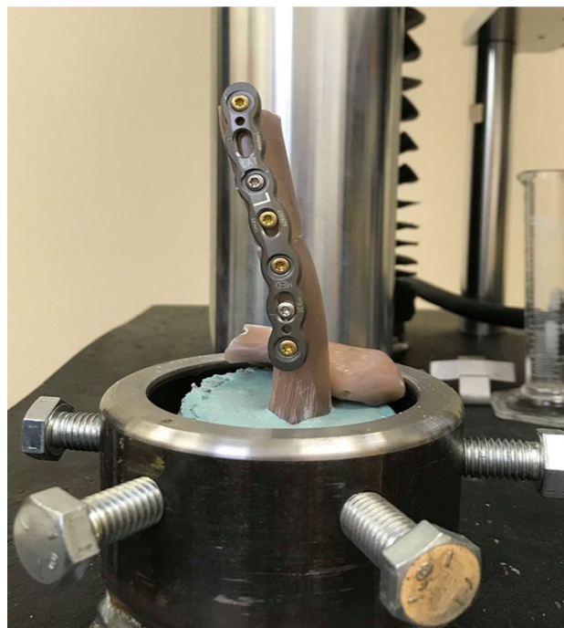
Fig. 4 Catastrophic failure of an anatomic superior pre-contoured locking plate after axial compression
