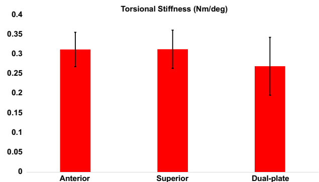
Fig. 7 Mean torsional stiffness values with 95% confidence intervals
