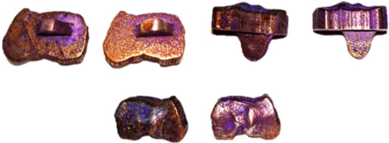
Fig. 4 Evidence of biofilm formation by crystal violet staining 1 week after incubation with S. aureus
