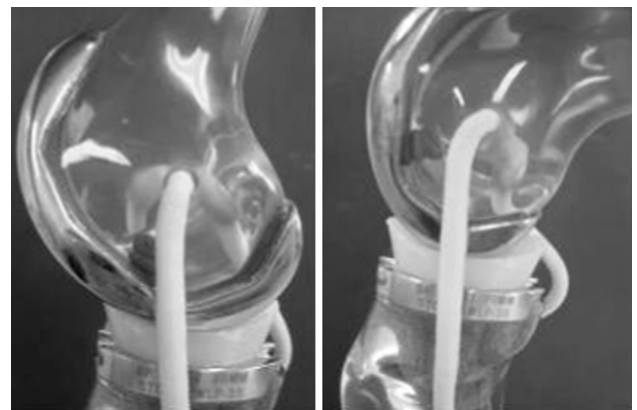
Fig. 2 Sagittal plane view of the LCS rotating platform TKA demonstrating femoral–tibial congruence at 30° (left, full contact) and 75° (right, partial contact) of flexion
