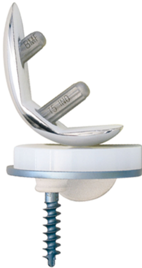
Fig. 1 The ALPINA ® UNI anatomic unicompartmental knee. For the femoral component, the internal surface is grooved and roughened for the cemented fixation and HA-coated for the cementless fixation. Two pegs at 30° angle increase the fixation and the stability of the femoral component. The tibial tray fixation and stability are ensured by 3 systems: a medial keel, a peg and an optional screw. Surfaces are grooved and roughened for the cemented fixation and HA-coated for the cementless fixation
