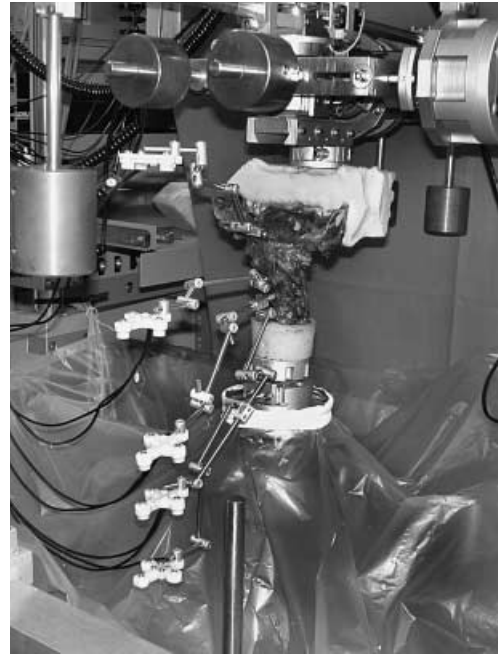
Fig. 2 Cervical human C0–C5 specimen fixed in the three-dimensional spinal loading simulator. Monosegmental motion of the segments C0–C2, C2–C3, C3–C4 and C4–C5 was measured using a non-contacting ultrasound motion analysis system
