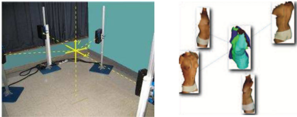
(a) System of four 3D optical digitizer to scan the patient. (b) Registering and merging of partial trunk surfaces.
