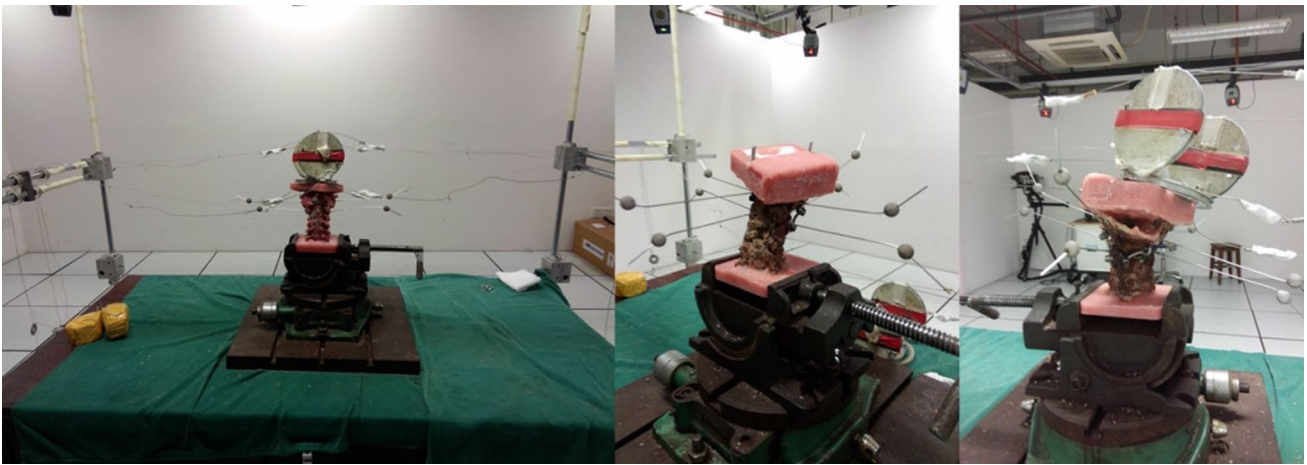
Fig. 4 Each specimen was fixed to the load frame of a custom-built six degree of freedom spine simulator, and a pure moment of 2.0 nm was applied to the cervical spine specimen using a testing system of cables and pulleys
