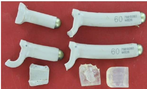
Fig. 7 Laboratory examination provided by Medtronic Co.: rod breakage near the centre of the C-shaped portion of each rod. Visual and optical examinations of the area of fracture initiation did not identify a pre-existing surface defect that could contribute to crack propagation
