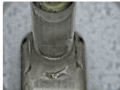
Fig. 9 Multiple witness marks around outside of the C shape suggests the MAS tulip head of the screw may have impinged against the C shape. This impingement condition may have created an undesired fulcrum, shifting the plane of maximum bending stress to a plane that is normal to the surface but intersects at the fulcrum
