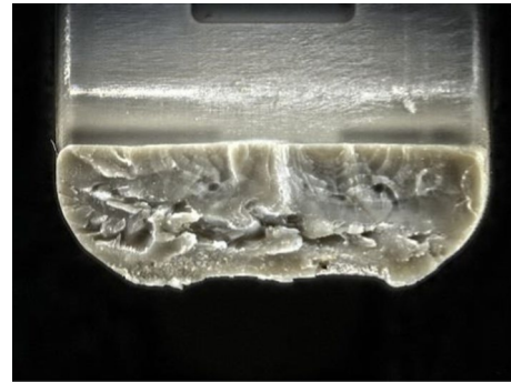
Fig. 8 Fracture surface examination identified a multi-modal fracture, with some evidence of convex-shaped progressive striations, initiating from the inside of the C shape and emanating outward, consistent with cyclic fatigue. The fatigue striations were followed by increased material disruption through the remaining cross-sectional area, consistent with overload
