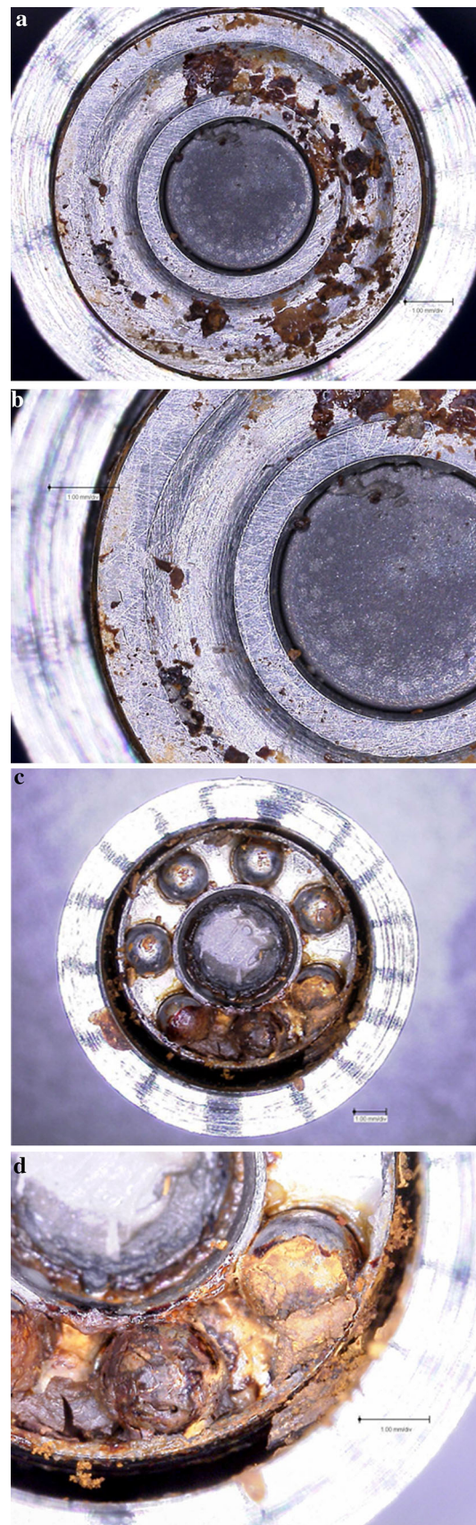
Fig. 8 a Microscopic image of the distal end of the magnet where thrust bearing articulates showing corrosive debris ( \times 50 magnification). b Microscopic image of the distal end of the magnet where thrust bearing articulates showing corrosive debris ( \times 100 magnification). c Microscopic picture of the thrust bearing showing signs of corrosion ( \times 50 magnification). d Microscopic picture of the thrust bearing showing signs of corrosion ( \times 100 magnification)
