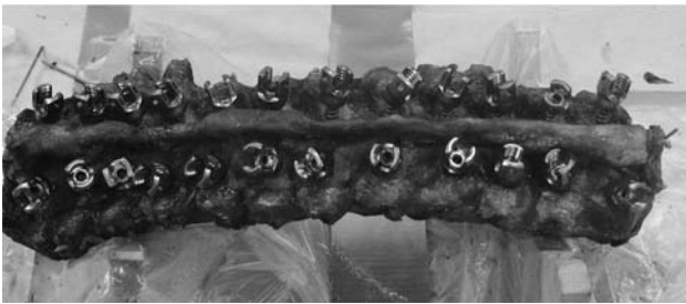
Fig. 3 Pedicle screws inserted on tapped (left) and untapped (right) pilot holes
