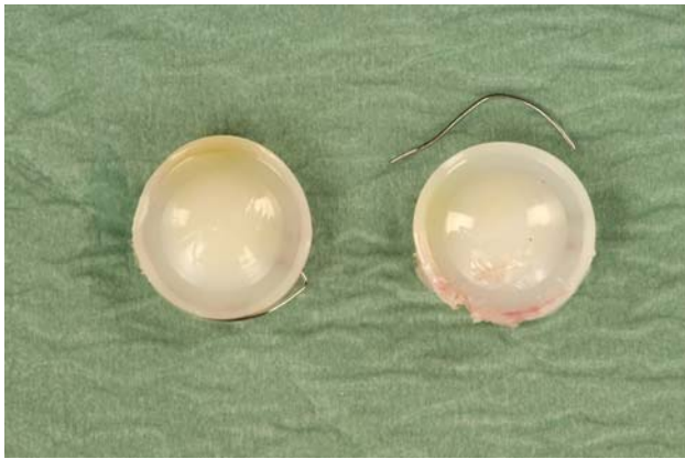
Fig. 2 Example of removed polyethylene core L4–5 ( left ) and L5–S1 ( right ) (6.5 years after insertion) with a fracture of the metal wire and damage of disc prosthesis
