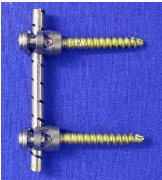
Fig. 1 The dynamic fixator tested in this study consisted of tangoRS polyaxial pedicle screws and flexible spiral-shaped rods. The same screws but solid rods (not shown) were used in case of the rigid fixator
