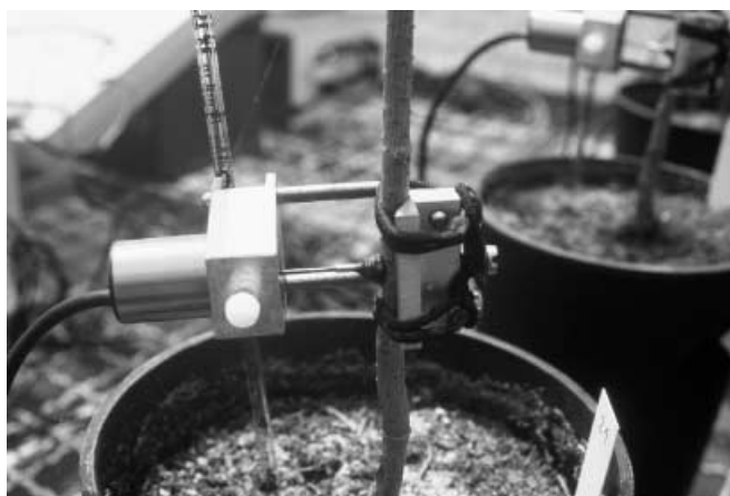
Fig. 1 Detail of the attachment of linear variable differential transformer sensors on the stem of Pinus pinea (stone pine) plants
