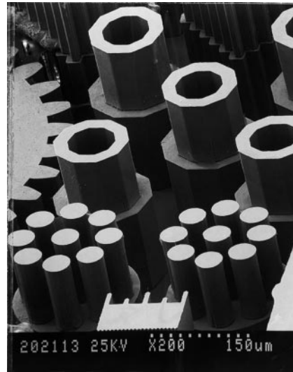
Fig. 2. LIGA with two, aligned X-ray masks
