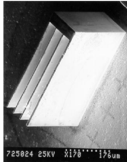
Fig. 4. A 350micron tall metal structure, with the thinnest line being 3 micron in width, producing an aspect ratio of approximately 110:1
