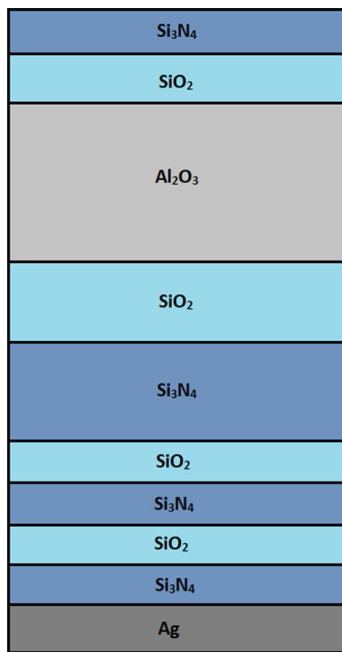
Fig. 20 Final design of the thin film material structure
