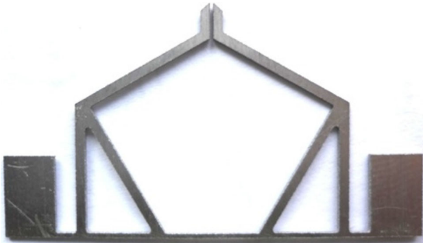
Fig. 10 The fabricated micro gripper frame using the wire-EDM method
