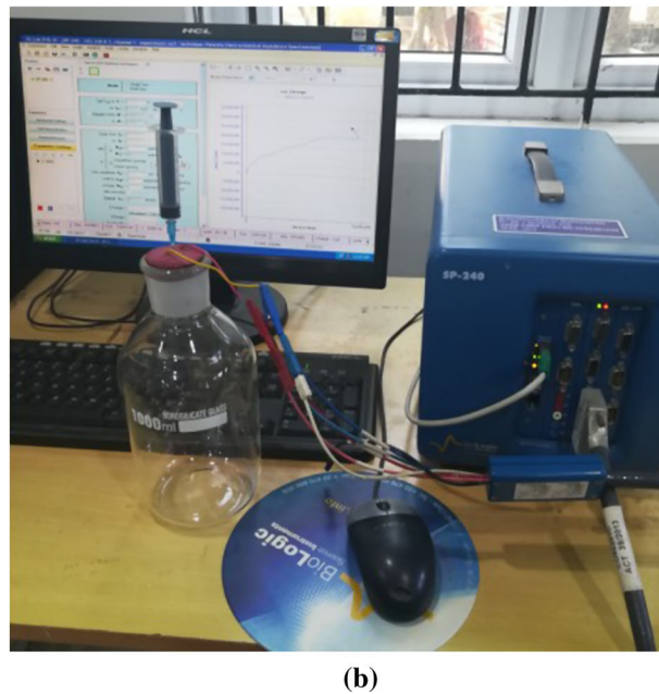
Fig. 4 a Schematic representation of benzene, butane and methane gas sensing experimental setup. b Experimental setup used for recording the performance of benzene, butane and methane gas sensor using electrochemical workstation
