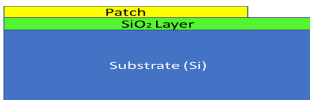
Fig. 2 View of micromachining part of the antenna
