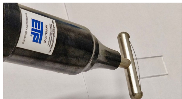
Fig. 4 Corona treatment on the PMMA samples just before adding the solvent to the samples
