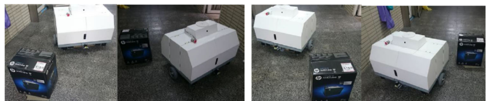
(a) Obstacle on the right (b) Avoiding the obstacle on the right (c) Obstacle on the left (d) Avoiding the obstacle on the left
