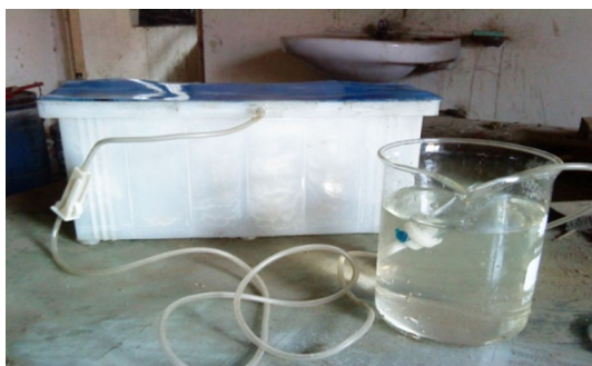
Fig. 22 An experimental set-up of hydrogen gas production by a PKL module
