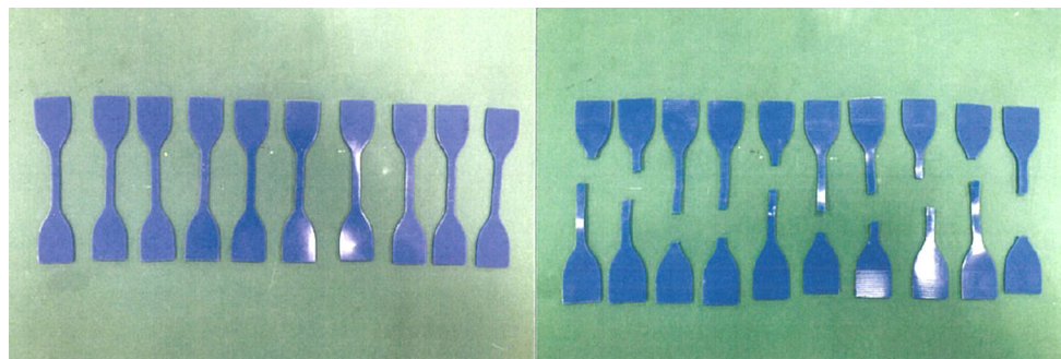
Fig. 4 ASTM D412-C tensile test specimens
