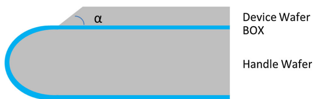
Fig. 1 Schematic view of a BSOI-wafer with shaped wafer edge, the angle \alpha should be between 30^\circ and 60^\circ
