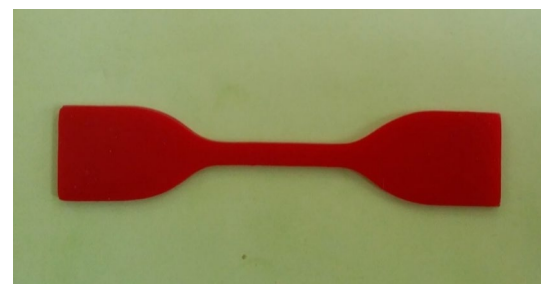
Fig. 3 Geometry of SR samples for uniaxial tensile testing
