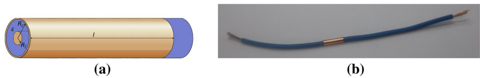
Fig. 4 a Scheme of the capacitance-coupling voltage sensor. b Photo of the sensor
