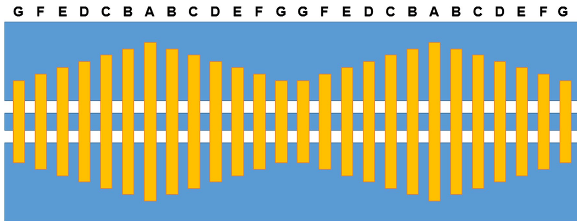
Fig. 9 Schematic view of the reconfigurable RF-MEMS-based phase shifter presented in Bakri-Kassem and Mansour (2013). The network employs RF-MEMS capacitive switches with 7 different lengths of
