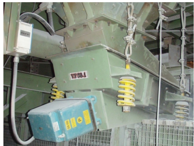
Fig. 4 Magnetic vibratory feeder, vibrating at 50 Hz
