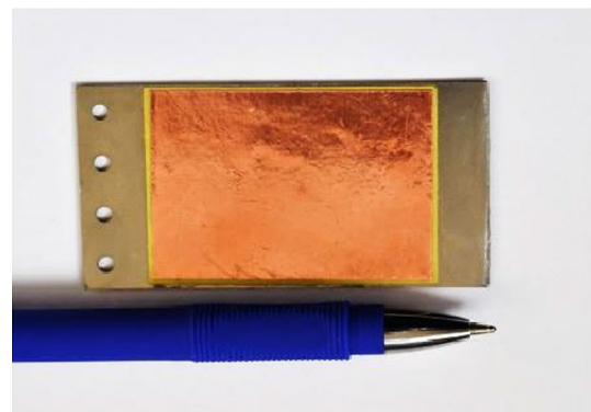
Fig. 6 Original shape of the bimorph cantilever beam
