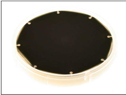
Fig. 4 Picture of a homogenous arrangement of nanostructures (typical black surface) on a 2 mm thick Si-wafer
