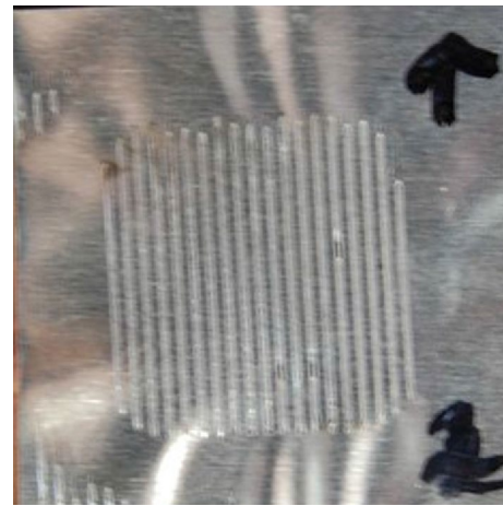
Fig. 3 An Al/Cu laser joining sample viewed from Al side
